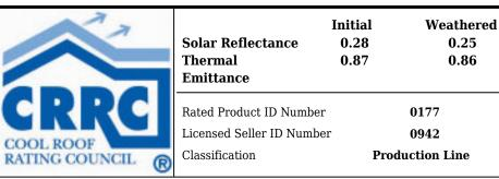
Cool Roof Rating Council ratings are determined for a fixed set of conditions, and may not be appropriate for determining seasonal energy performance. The actual effect of solar reflectance and thermal emittance on building performance may vary. Manufacturer of product stipulates that these ratings were determined in accordance with the applicable Cool Roof Rating Council procedures.
